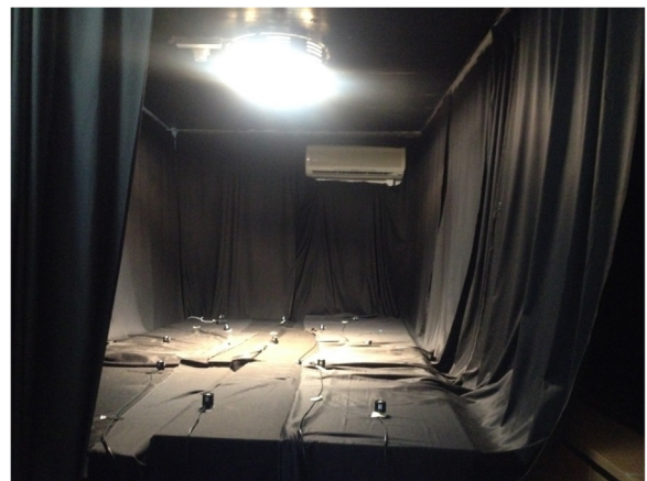
Fig. 2. The layout of the illuminance sensors.
