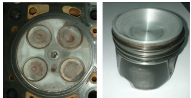
Fig. 1. Four valve heads with central spark plug (right) and modified pistons with enlarged bowl (left).
