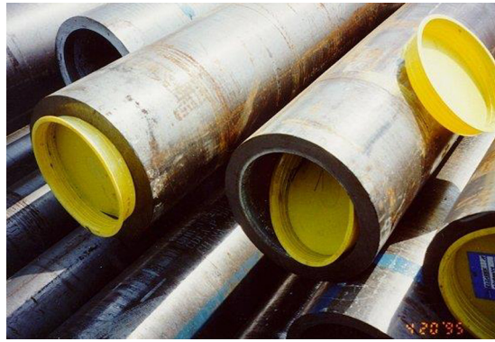
Fig. 1. Plastic caps cover at the end of the tube prior to shipment.
