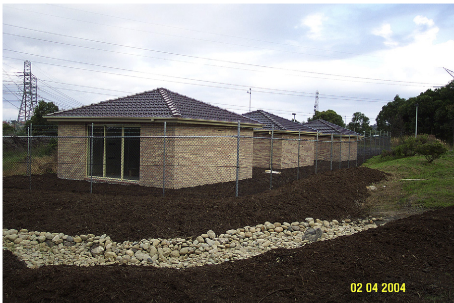
Fig. 1. Four thermal housing test modules using different wall systems on the Campus of The University of Newcastle, Australia.
