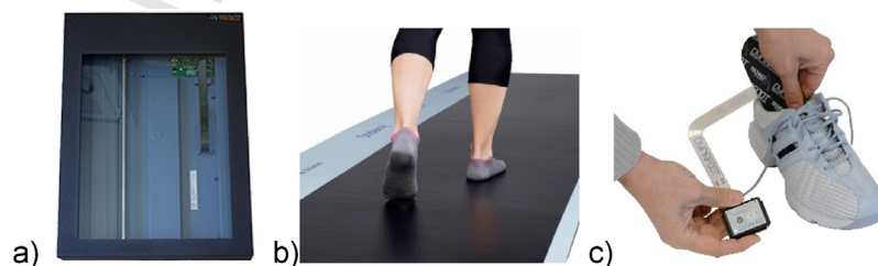
Fig. 1 – Plantar pressure measurement systems. (a) Optical pedo-barographs [8]. (b) Pressure platform [9]. (c) Instrumented footwear [10].
