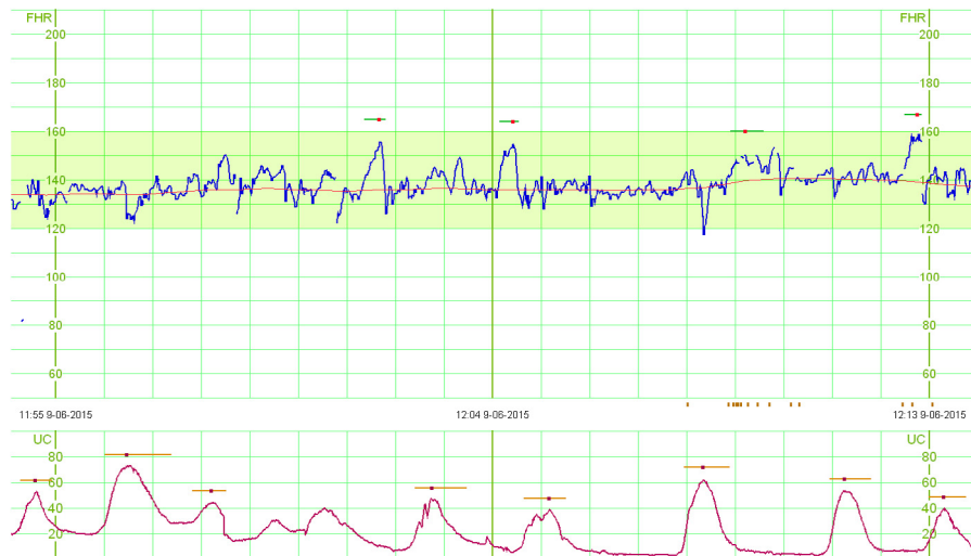
Fig. 1 – Computer screen from a fetal monitoring system with cardiocotographic trace comprising two signals: Fetal Heart Rate – FHR (upper) and Uterine Contractions – UC (lower). Graphical marker of detected uterine contraction is formed by horizontal line corresponding to contraction duration, and vertical one indicating its peak.
