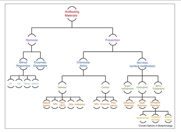
A schematic overview of mechanisms for developing antifouling materials. On the left are approaches to remove accumulated biomass. On the right are approaches to prevent the adsorption in advance.
