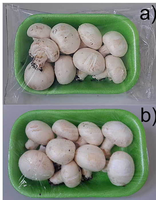
Fig. 1. Button mushrooms packaged in the bionanocomposite-based laminate/EPS tray (a) and in the conventional PVC stretchable/EPS tray configuration (b) tested in this study.
