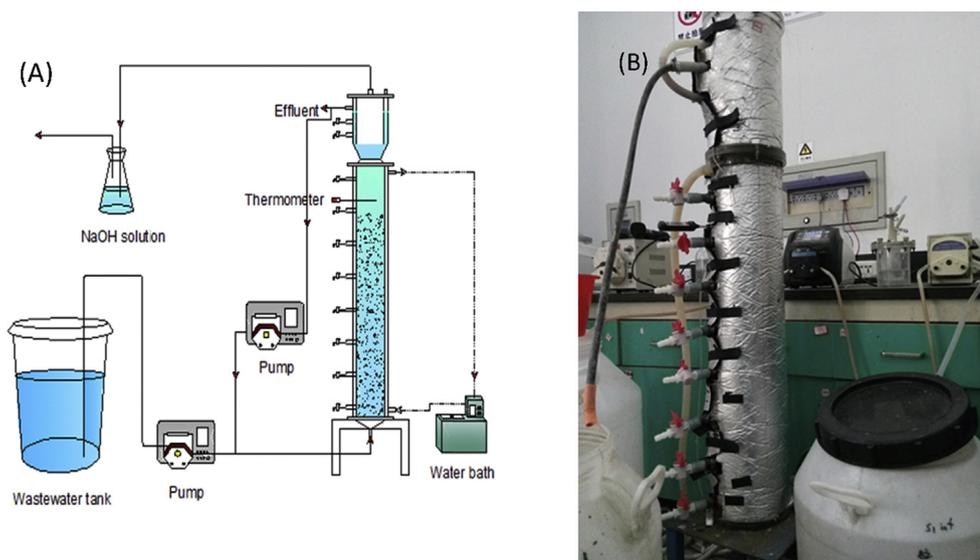
FIG. 1. Schematic diagram (A) and photograph (B) of the anammox-UASB system.
