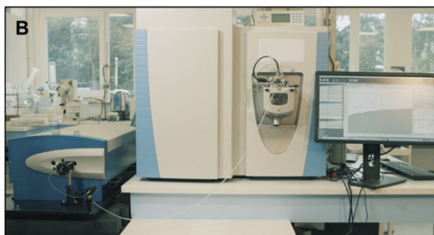
Fig. 1. A) Schematic representation of the SpiderMass system showing the connection between the laser, the mass spectrometer and sampling probe. B) Picture of one system with the laser system on the left with the fiber and the sampling probe in front of it, the mass spectrometer and its computer on the right and the transfer tubing linking both parts.
