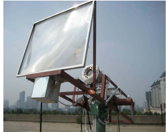
Fig. 2. Photo of two-axis tracking solar powered thermoacoustic engine.
