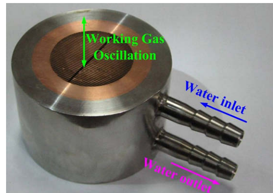
Fig. 3. Photo of the cooling heat exchanger.
