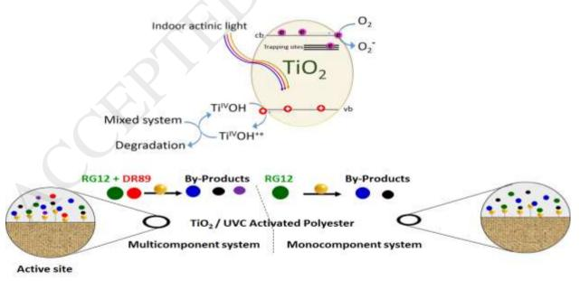
Contribution of Reactive species for removal of textile effluent with photocatalysis under UV and visible lights
