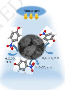
Schematic representation of photocatalytic degradation of PNP with ZnNiAl-LDO photocatalyst prepared by microwave-assisted method under visible-light irradiation.
