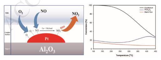
Catalytic oxidation of NO to NO<sub>2</sub> over Pt/Al<sub>2</sub>O<sub>3</sub> catalyst at nitric acid plant conditions
