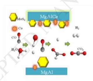
The more and smaller-sized  $MoS_2$  which is active for the water gas shift reaction was formed on the Co-Mo/Mg(Al)O-Ce(5%) catalyst than Co-Mo/Mg(Al)O catalyst.
