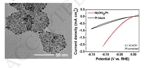
The Pt/Ni(OH)<sub>2</sub> hybrid nanostructures showed enhanced electrocatalytic activity toward hydrogen evolution reaction in alkaline condition likely due to synergetic effect of Ni(OH)<sub>2</sub> and Pt.
