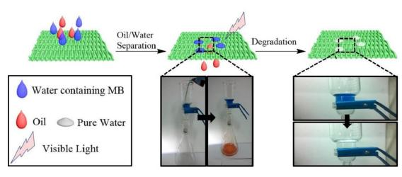
A dual-layer copper mesh consists of a superhydrophobic Ag-coated mesh and a photocatalytic GO/AgBr-coated mesh was fabricated for water purification via separation of insoluble oil from water and successively photodegradation of soluble organic dyes.
