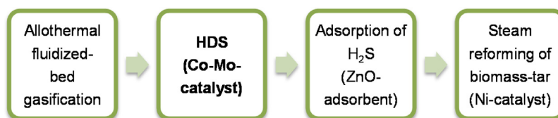
Fig. 1. Scheme of the discussed gas cleaning process.
