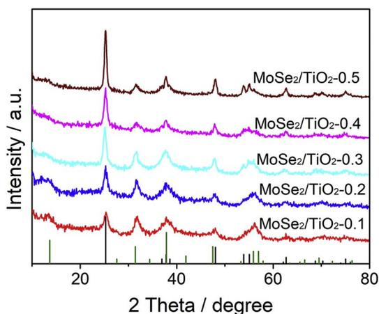
Fig. 1. Powder XRD patterns of  $\text{MoSe}_2/\text{TiO}_2\text{-X}$  ( $X = 0.1, 0.2, 0.3, 0.4$  and  $0.5$ ). The bottom bars present the standard diffractograms of  $\text{TiO}_2$  (black, JCPDS card no. 21-1272) and  $\text{MoSe}_2$  (green, JCPDS card no. 29-0914). (For interpretation of the references to colour in this figure legend, the reader is referred to the web version of this article.)
