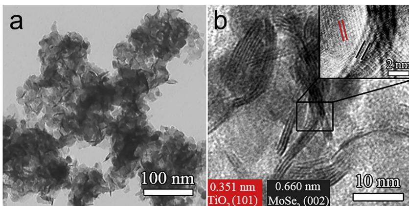
Fig. 2. (a) TEM and (b) HRTEM images of  $\text{MoSe}_2/\text{TiO}_2\text{-0.3}$  solid composite.
