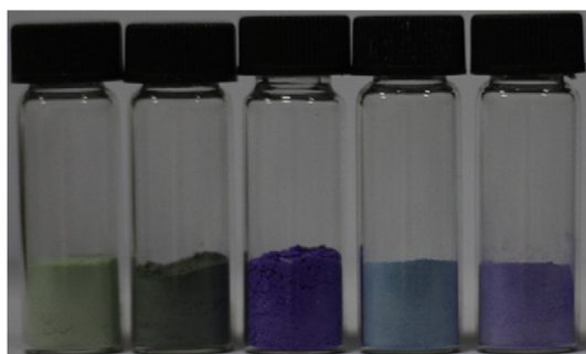
Fig. 2. The colors of [Cu-Imace-H][X]. From left to right: X^- = \text{Cl}^-, \text{Br}^-, \text{HSO}_4^-, \text{NO}_3^-, \text{and } \text{BF}_4^- .
