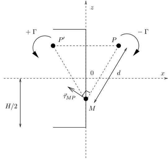
Fig. 1. Location of the vortex center  $P$  respecting to the wall.
