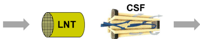
Fig. 1. Schematic representation of catalyst configuration for the H 2 S suppression experiment.
