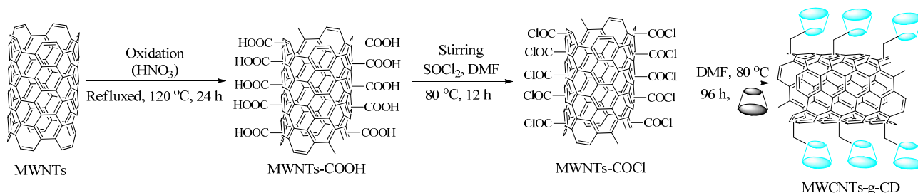
Scheme 1. Schematic diagram of the MWCNTs-g-CD preparation process.
