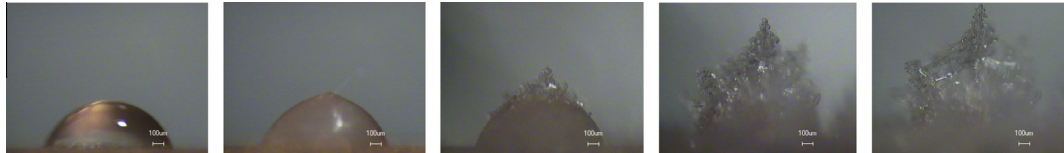
Fig. 2. Real process of frost crystal growth on the frozen water droplet surface.
