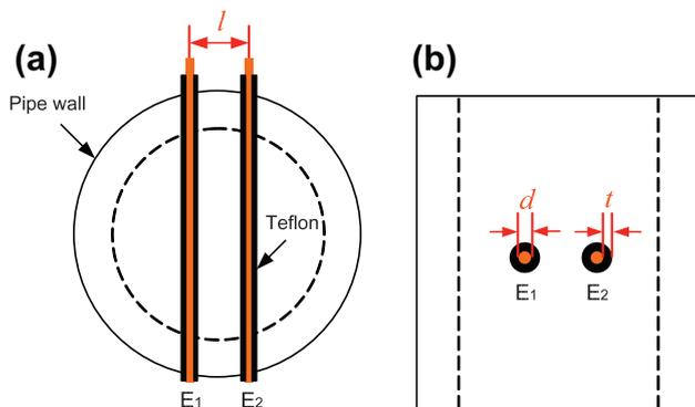
Fig. 1. The sketch of the PWCP: (a) radial section of the pipe and (b) axial section of the pipe.
