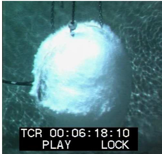
Fig. 1. Single frame of video footage provided by SERCEL of GGun150 fired at 138 bar (2000 psi).
