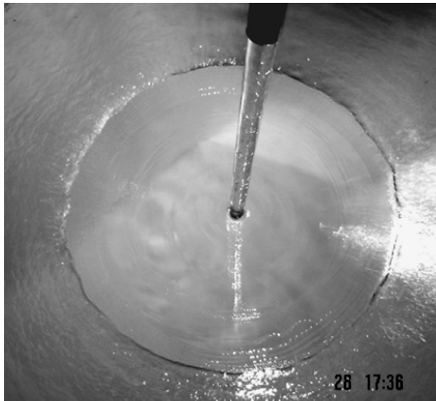
Fig. 1. Circular hydraulic jump due to a normal impinging circular liquid jet with a volume flow rate of water, Q = 1 \times 10^{-4} \text{ m}^3/\text{s} , nozzle diameter, d = 8.8 \text{ mm} .
