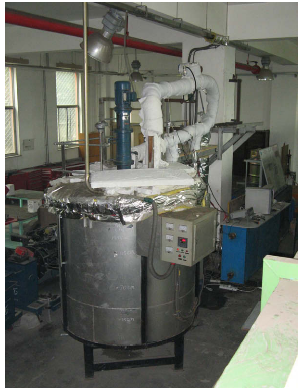
Fig. 2. Experimental system picture for forced convection heat transfer with molten salt.
