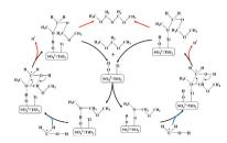
Reaction mechanism for the synthesis of  $PODE_n$  on Brønsted and Lewis acid sites.
