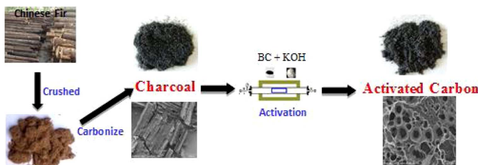
Fig. 1. Schematic illustration of the complete synthesis route of the AC samples.
