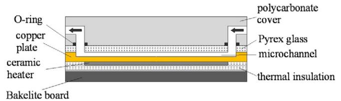
Fig. 2. Schematic diagram of the test section.
