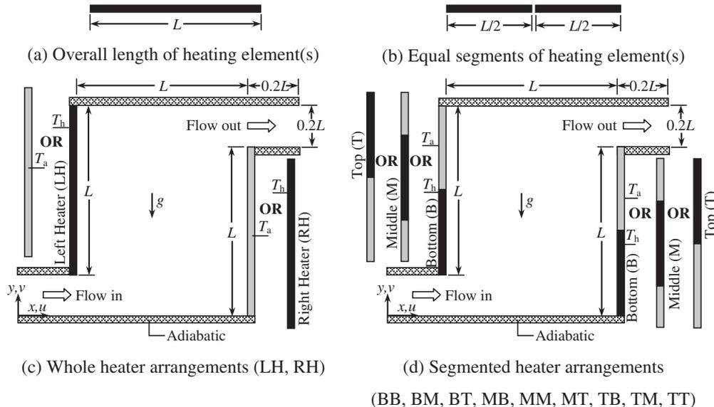
Fig. 1. Schematic arrangement of heating element in a ventilated enclosure.
