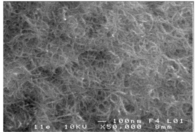
Fig. 1. SEM picture taken from dried nanofluid with lignin as surfactant with 0.55% in volume fraction of nanotubes.
