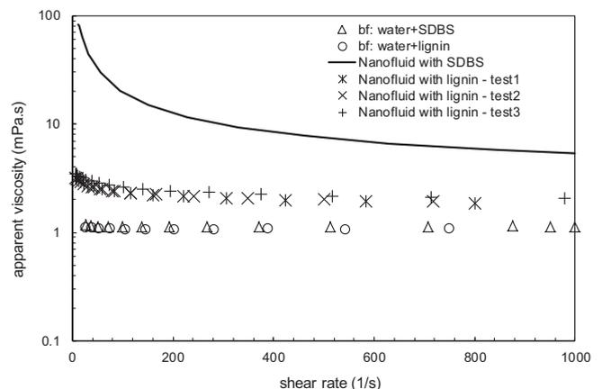
Fig. 2. Viscosity of nanofluids and base fluids versus shear rate – Influence of surfactant.
