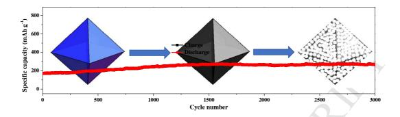
3D porous carbon material derived from metal-organic frameworks exhibits ultrafast sodium storage ability owing to high pseudocapacitive contribution.
