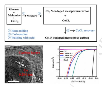
Co-entrapped, N-doped mesoporous carbon was synthesized via combination of hand milling and carbonation.  $CoCl_2$  was utilized as the template, which could be removed and recovered. The obtained catalyst exhibits excellent performance for hydrogen evolution reaction in acidic media.
