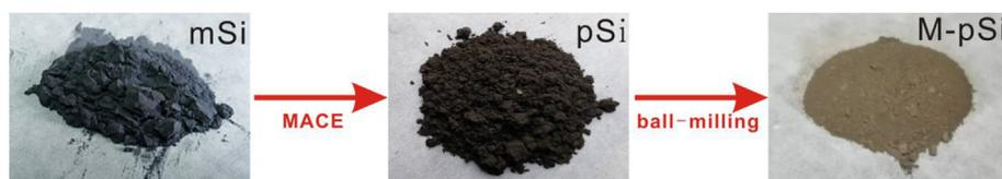
Fig. 1. Synthetic route of M-pSi from mSi through MACE method and ball-milling.
