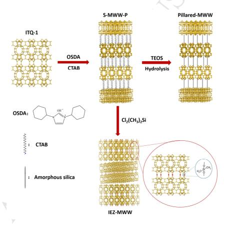
In this study, IEZ-MWW and Pillared-MWW were obtained by the post-synthesis modifications of the swollen multilamellar MWW precursor (S-MWW-P), which have better catalytic performances than 3D-MWW and ZSM-5 in the condensation of cyclohexanone with glycol or benzaldehyde with 1-pentanol.
