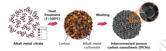
One-step synthesis of interconnected porous carbon nanosheets with controllable pore size via self-templating process for electrochemical capacitors
