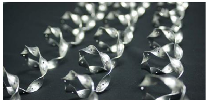
Fig. 1. Photograph of perforated helical twisted-tapes (P-HTTs): (a) a perforated helical twisted-tape (P-HHT) modified from a straight perforated twisted-tape (PTT) and (b) isometric view of perforated helical twisted-tape.
