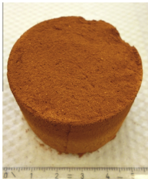
Fig. 1. Photograph of a subcritically dried base–acid catalyzed resorcinol–formaldehyde (RF) aerogel synthesized.
