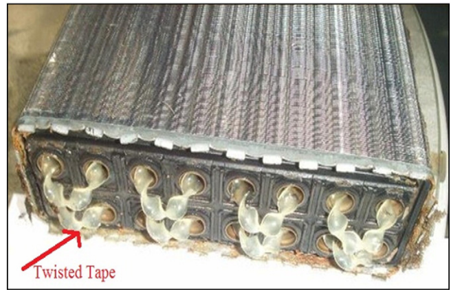
Fig. 2. TT insert into the industrial heat exchanger (car radiator).
