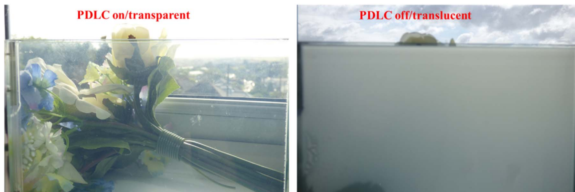
Fig. 3. Photographs of PDLC glazing for its switch on and switch off states.
