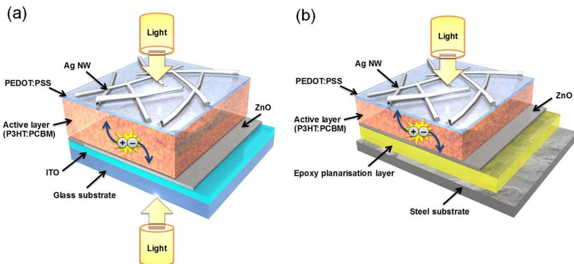
**Fig. 1.** Schematic of the (a) semi-transparent OPV where photocurrent can be achieved bifacially and (b) of the OPV manufactured onto steel. Planarization of the underlying substrate is imperative to ensure no electrical shorts are present.
