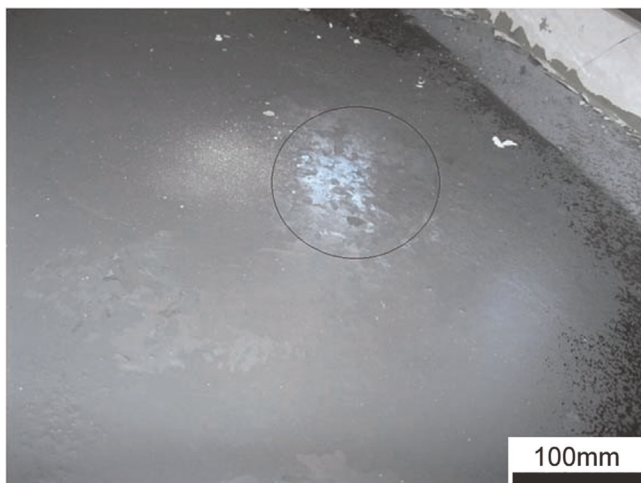
Fig. 1. Optical photo of the top surface of reference ML silicon ingot (ingot A) from an oblique angle. Sub-grains could be observed, as indicated by the circle.
