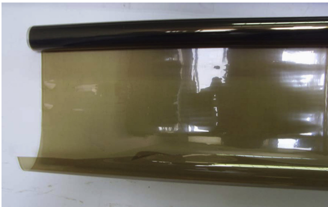
Fig. 1. Thermal-stable PET film covered with VO 2 .
