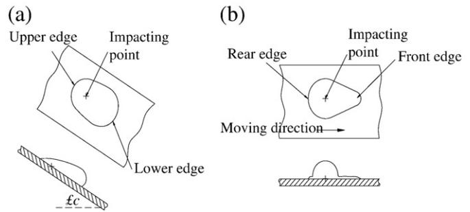
Fig. 1. Sketch of the geometry of drop spreading film (a) on an inclined surface (b) on a moving surface.
