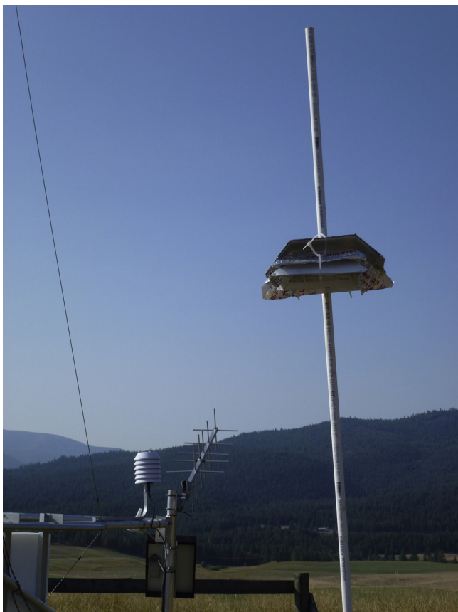
Fig. 1. Inexpensive solar radiation shield (radshield) mounted on a PVC pole adjacent to the Ninemile RAWs station, Montana.
