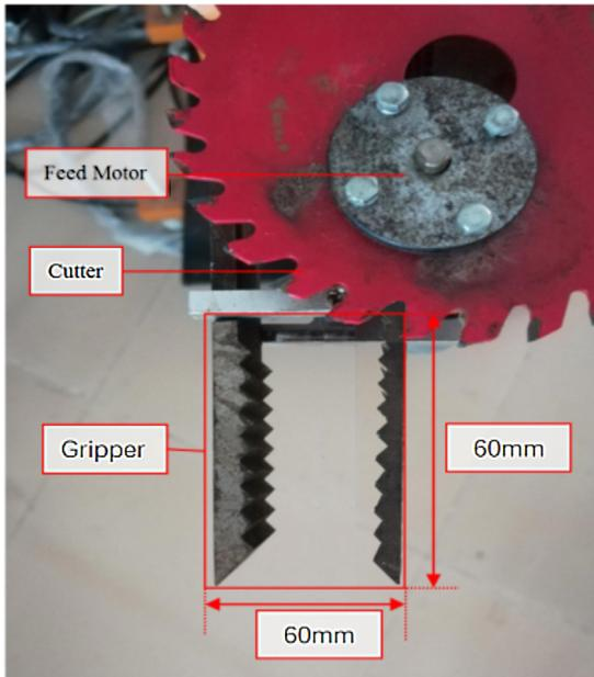
Fig. 1. End effector structure of litchi picking robot.
