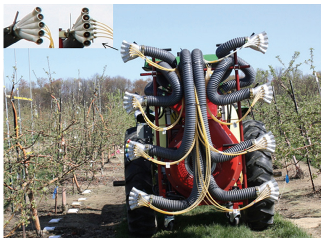
Fig. 1. An intelligent sprayer with four five-nozzle manifolds on both side of the sprayer (Chen et al., 2013).
