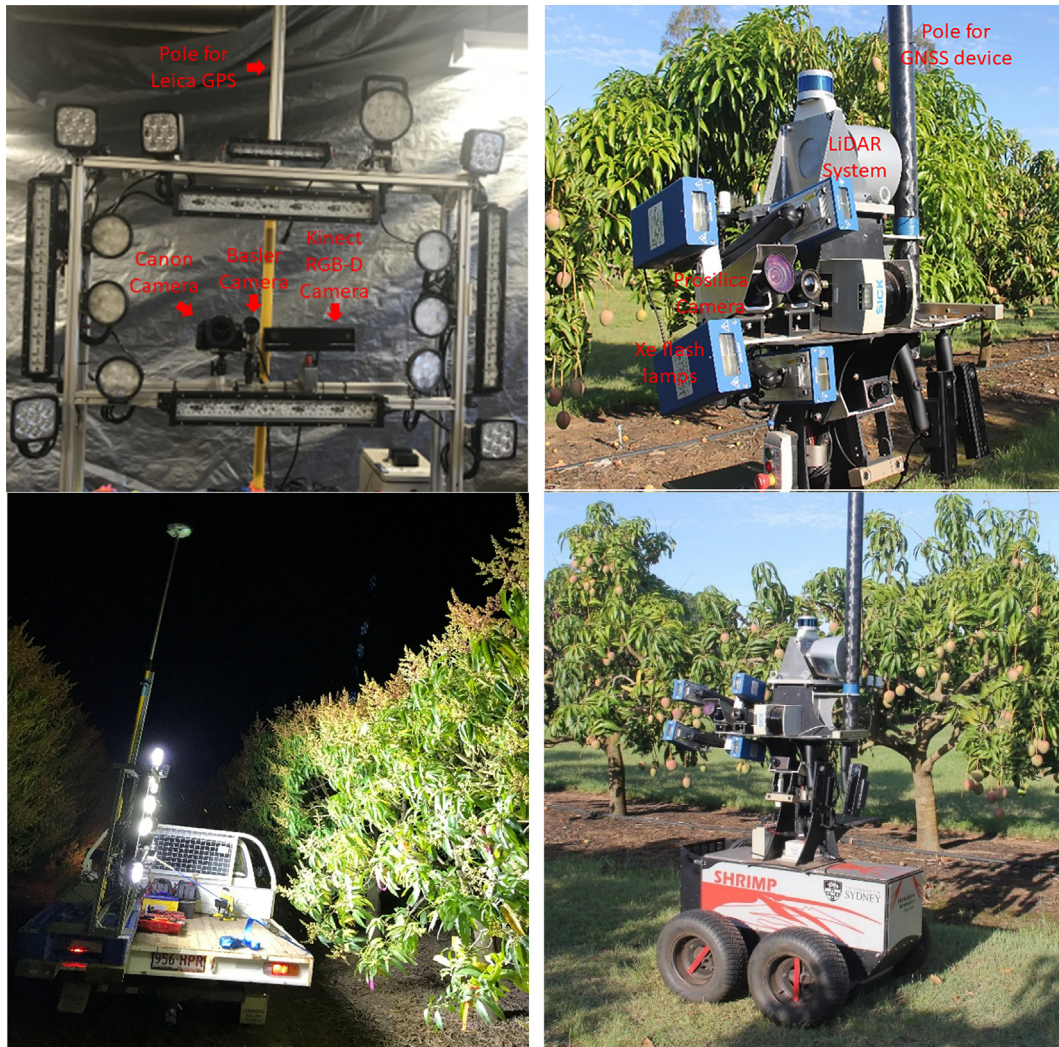
Fig. 1. The two systems used in the imaging of mango tree flowering: Platform A (left panels) and B (right panels), showing sensors on top row and platforms on bottom row.
